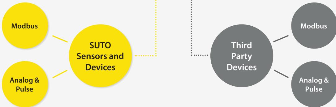
SUTO SDI and Modbus/RTU sensors as well as analog sensors can be connected to the S4M SaaS within minutes. To connect the Modbus/RTU sensors properly on an RS 485 bus system, it's recommended to daisy-chain the sensors to one of the inputs. For this purpose, SUTO offers a RS 485 splitter to simplify the connection.
