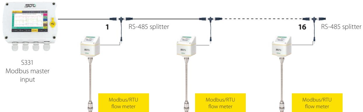
Flow meters can be easily integrated into a Modbus/RTU network (daisy chain)
